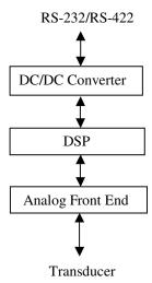
Fig. 4: Hardware structure
